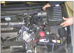
8. Remove the complete air box assembly from the vehicle.
