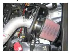
25. Install the  $K\&N^{\otimes}$  air filter and secure with the provided hose clamp.
