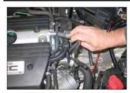
Release the spring clamp which secures the crank case vent hose to the valve cover and then unhook crank case vent hose from the valve cover as shown
