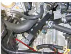
13. Using the provided bolt, secure the intake tube mounting bracket (070124) to the heater hose mounting bracket and thermostat housing from step #12.
