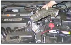
5. Remove the stock intake tube from the vehicle.
