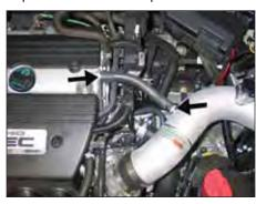
24. Install the provided crankcase vent hose onto the valve cover port and then to the vent fitting on the  $K\&N^{\otimes}$  intake tube.
