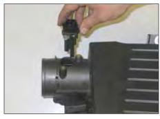
21. Remove the mass air sensor from the stock air box.
