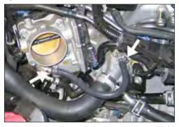
11. Install the provided coolant bypass hose onto the throttle body and thermostat housing and secure with the provided hose clamp.
