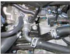
12. Remove the bolt shown that secures the heater hose mounting bracket to thermostat housing.
