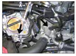
10. Release the two spring clamps securing the coolant bypass hoses to the throttle body and thermostat hosing, then remove the bypass hose assembly from the vehicle.
