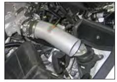
19. Install the K&N<sup>®</sup> intake tube into the silicone hose at the throttle body and align with the mounting bracket. Secure with the hose clamp and provided hardware.
