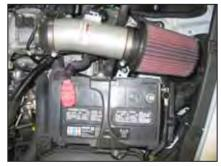
22. Reinstall the battery and secure with the hold down bracket. Reconnect the positive battery cable.
