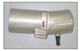
16. Install the  $\frac{1}{4}$  " NPT fitting into the K&N  $^{\otimes}$  intake tube as shown.
