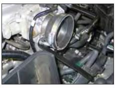
15. Install the silicone hose (084093) onto the throttle body and secure with the provided hose clamp.
