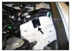
10. Remove the airbox mounting bracket bolt shown.
