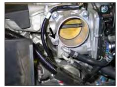
8. Remove the front lower throttle body bolt shown. **NOTE: This bolt will be reused in the next step.**
