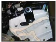
11. Install the heat shield mounting bracket (070116) onto the airbox mounting bracket and secure with the provided hardware.
