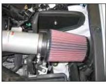
21. Install the K&N<sup>®</sup> air filter onto the intake tube and secure with the provided hose clamp.
