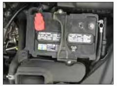
1. Turn off the ignition and disconnect the negative battery cable.
