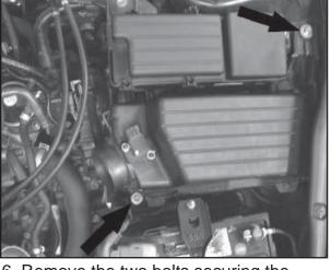
6. Remove the two bolts securing the stock air box to the vehicle.
