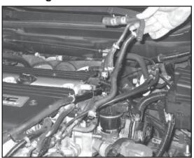
10. Remove the stock coolant hose assembly from the vehicle.
