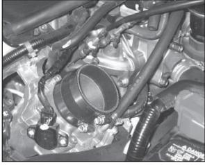
12. Install the provided silicone hose (#08440) onto the throttle body. Secure with the provided hose clamp as shown.
