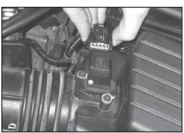
2. Depress the locking tab and remove the mass air sensor connector. Remove the clips securing the mass air sensor harness to the stock air box and intake tube.
