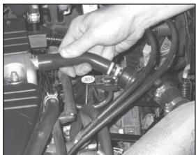
27. Install the crank case chamber assembly onto the K&N intake tube and valve cover. Secure with the provided hose clamp.
