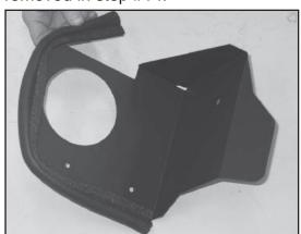
16. Install the provided edge trim onto the heat shield as shown.
