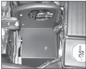
18. Install the heat shield assembly with the provided hardware as shown.
