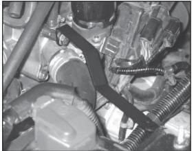
13. Install intake tube bracket (#06498) onto the thermostat housing with the provided hardware as shown.
