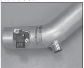
21. Install the mass air sensor into the K&N intake tube with the provided hardware as shown.
