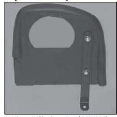
17. Install "L" bracket (#06499) onto the heat shield with the provided hardware as shown.
