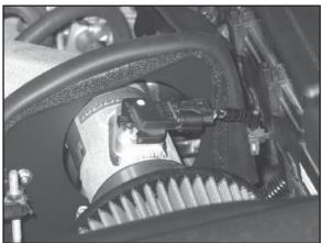
30. Re-connect the mass air sensor connector as shown.
