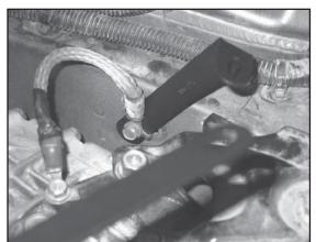
15. Install angled "L" bracket (#06497) onto the frame rail. Secure the "L" bracket and ground strap using the bolt removed in step #14.
