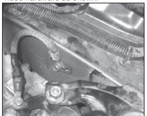
14. Remove the bolt securing the ground strap to the frame rail.
