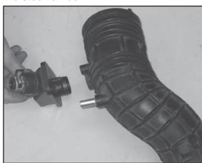
20. Depress the spring clamp and remove the crank case vent chamber from the stock intake tube.
