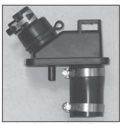
23. Install the provided silicone hose (#084074) onto the stock crank case vent chamber. Secure with the provided hose clamps as shown.
