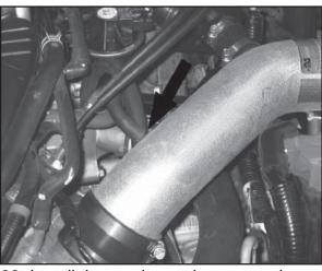
28. Install the stock vent hose onto the K&N intake tube as shown. Secure with the provided hose clamp.
