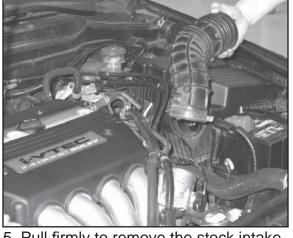
5. Pull firmly to remove the stock intake tube from the air box. Remove the intake tube from the vehicle.
