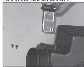
19. Remove the mass air sensor from the stock air box.
