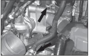
9. Depress the spring clamps on the stock coolant hose at the throttle body and thermostat housing.
