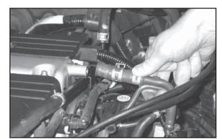
8. Depress the spring clamp and remove the crank case vent hose from the valve cover.
