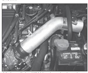
22. Install the K&N intake tube into the silicone hose at the throttle body and align with the tube mounting bracket installed in step # 13. Secure with the provided hardware and hose clamp.
