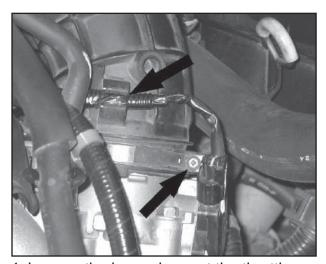
4. Loosen the hose clamp at the throttle body and unclip the throttle position sensor harness from the stock intake tube.
