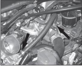
11. Install the supplied coolant hose onto the thermostat housing and throttle body. Secure with the provided clamps as shown. Note: Replace any coolant recovered during hose removal by replenishing the recovery tank. Some trimming of the coolant hose may be necessary.
