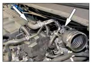
7. Release the spring clamps securing the crank case vent hose connections to the valve cover and intake hose, and then disconnect crank case vent hose connections.
