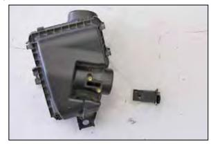
19. Remove the two screws securing the mass air sensor and then remove the mass air sensor from the factory air box.
