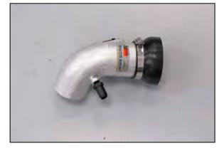
24. Install the provided silicone hose (084093) onto the Intake tube as shown and secure with the provided hose clamp.
