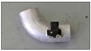
20. Install the mass air sensor into the  $K\&N^{\circledast}$  intake tube and secure with the provided hardware.
