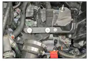
14. Install the bracket assembly onto the front air box mount as shown.
