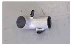
23. Install the provided vent fitting into the K&N $^{\mbox{\tiny \$}}$  tube as shown.
