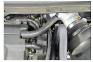
29. Install the provided crank case vent hose onto the vent port of the valve cover and to the fitting installed into the K&N<sup>®</sup> intake tube.
