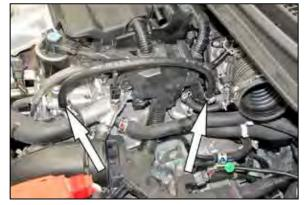
9. Install the provided coolant by-pass hose and secure with the provided hose clamp.
