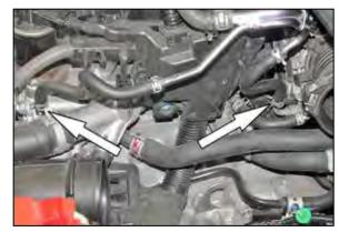
8. Release the spring clamps securing the coolant by-pass hose connections to the engine and then disconnect the coolant by-pass hose and remove the by-pass hose/crank case vent pipe assembly. **NOTE: be sure the engine is cool before attempting to remove the coolant by-pass hose. Be sure to collect any lost coolant and replenish into the cooling system once the install is complete.**
