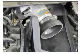
25. Install the intake tube into the silicone hose at the throttle body as shown. Do not tighten the hose clamp at this time.
