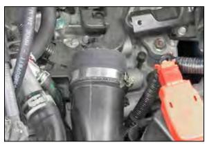
12. Install the provided silicone hose (08190) onto the fresh air duct and secure with the provided hose clamp.
