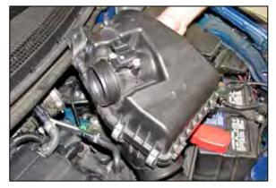
6. Disconnect the mass air sensor electrical connection and then remove the complete air box assembly.
