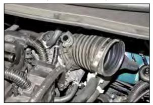
10. Loosen the hose clamp securing the intake hose to the throttle body and remove the intake
