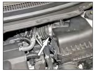
2. Loosen the hose clamp securing the intake tube to the air box and then disconnect the tube from the air box.
