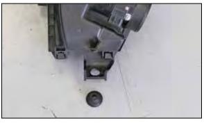
15. Remove the mounting grommet from the air box as shown.
