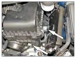
4. Remove the two bolts retaining the air box.
