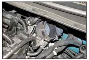
11. Install the provided silicone hose (084016) onto the throttle body and secure with the provided hose clamp. R.
