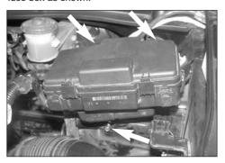
13. Unclip the fuse box (3 places) and lift the fuse box upwards as shown.
