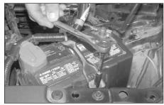
18. Move the battery back into position and secure it with the battery hold down bracket as shown.
