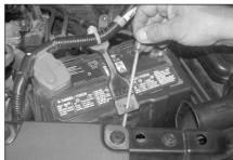
10. Loosen the battery hold down bracket and shift the battery to the left to gain clearance for the removal of the resonator.
