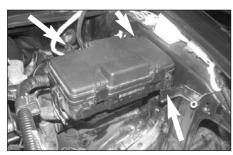
17. Install the fuse box back onto the stock bracket as shown.
