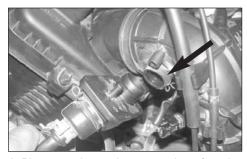
3. Disconnect the crank case vent hose from the stock intake tube as shown.
