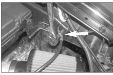
33. Reconnect the ground cable to the inner fender as shown.
