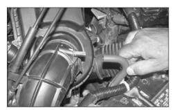
2. Disconnect the vent hose from the stock intake tube as shown.
