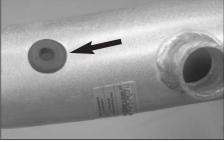
24. Install the provided grommet into the hole on the K&N Typhoon intake tube as shown.
