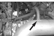
29. Reconnect the vent hose to the vent on the K&N Typhoon intake tube as shown.
