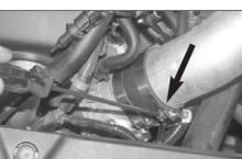
28. Tighten the hose clamp at the throttle body as shown.
