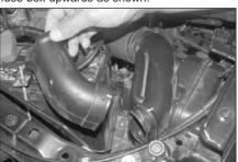
14. Remove the resonator inlet as shown.
