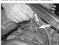
11. Loosen and remove the battery ground at the inner fender as shown.
