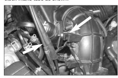
4. Unclip the cruise control cable and the throttle cable from the stock intake tube as shown.
