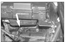
20. Remove the bolt on the lower fuse box
