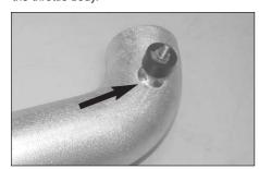
23. Install the rubber mounted stud into the threaded boss on the K&N Typhoon intake tube as shown.
