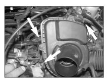
7. Loosen the three bolts that secure the air cleaner assembly to the engine as shown
