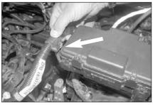
19. Clip the wire harness onto the stock fuse box bracket as shown.
