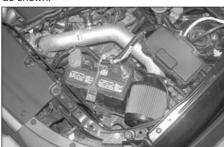
34. Reconnect the negative battery cable and double check that everything is tight and properly positioned before starting the vehicle.
