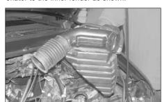
16. Remove the resonator as shown.
