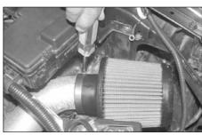
32. Install the K&N Air Filter onto the K&N Typhoon intake tube and secure with the provided hose clamp as shown.
