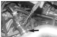
30. Install the provided silicone hose and hose clamps onto the crank case vent, then, connect the other end to the vent on the K&N Typhoon intake tube as shown.
