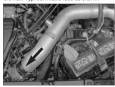
25. Slide the tube into the silicone hose as shown, but do not tighten at this time.
