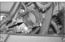
22. Install the silicone hose and hose clamps onto the throttle body and tighten the hose clamp on the throttle body.
