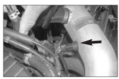
31. Install the air temperature sensor into the grommet on the K&N Typhoon intake tube as shown.
