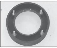
15. Install the four 6mm studs into the air filter adapter; threading them down until they bottom into the insert. tighten fingertight.
