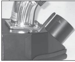
20. Install mounting bracket (#06507) onto the heat shield using the provided hardware as shown.
