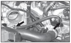
12. Install the provided bypass hose onto the throttle body and intake manifold ports. Secure with the provided hose clamps.
