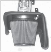
21. Install the K&N air filter onto the air filter adapter and secure with the provided hose clamp.
