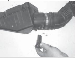
13. Remove the two screws that secure the mass air sensor to the upper air box, then remove the mass air sensor as shown.
