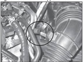
3. Release the spring clamp, then disconnect the EVAP canister hose from the intake tube as shown.
