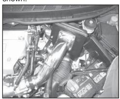
25. Install the intake assembly into the silicone hose at the throttle body and align the mounting bracket with the air box mounting stud. Secure the intake assembly with the provided hose clamp and hardware. Secure the fresh air tube to the heat shield with the hose clamp.
