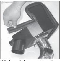
19. Install the provide edge trim onto the heat shield as shown.
