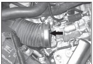
24. Install the provided hose clamp onto the stock fresh air supply hose as shown.
