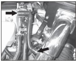
29. Install the crank case vent hose assembly onto the valve cover port and intake tube port as shown.
