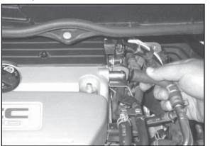
9. Release the spring clamp that secures the crank case vent hose to the valve cover, then disconnect the crank case vent hose from the valve cover.
