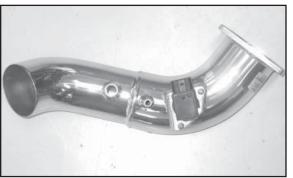
14. Install the mass air sensor into the K&N intake tube and secure with the provided hardware.
