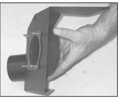
17. Install the air filter adapter into the heat shield as shown. Place the remaining gasket onto the exposed studs as shown.
