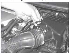
2. Disconnect the mass air sensor electrical connection. Un-clip the mass air sensor wiring harness from the upper air box.
