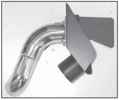
18. Install the K&N intake tube onto the exposed studs and secure with the provided hardware.
