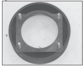
16. Place one of the provided gaskets onto the air filter adapter as shown.
