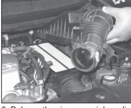
5. Release the six upper air box clips, then remove the upper air box and intake tube assembly as shown.
