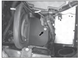
14. Install the heat shield assembly into the vehicle and secure to the engine mount using the bolt removed during step #10.
