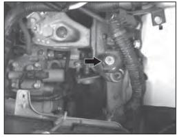
10. Remove the transmission mount bolt shown.
