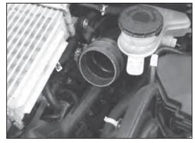
16. Install the provided silicone hose (08711) onto the turbo inlet tube and secure with the provided hose clamp.
