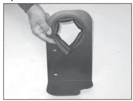
11. Install supplied short edge trim into the hole of the heat shield as shown.
