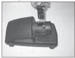
18. Remove the two mass air sensor retaining bolts and the remove the mass air sensor from the stock air filter housing.
