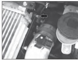
20. Install the K&N® intake tube into the silicone hose at the turbo inlet tube and align so the mounting bracket lines up with the turbo inlet mounting location. Secure the intake tube with the hose clamp and hardware provided.
