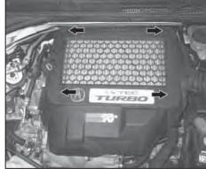
2. Loosen the four quarter turn fasteners that attach the engine cover and lift off the engine cover.
