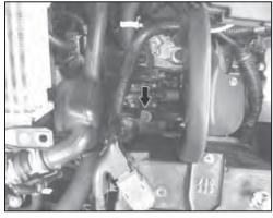
15. Secure the heat shield mounting bracket to the lower airbox mounting tab using the bolt removed in step #7.
