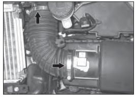
4. Loosen the two hose clamps that secure the intake tube to the airbox and turbo inlet tube.
