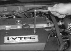
25. Reinstall the engine cover and secure with the original hex bolts as shown.
