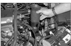
11. Remove the air inlet duct as shown.
