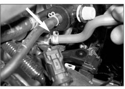
12. Remove the stock IA bypass control thermal valve vent hose as shown.
