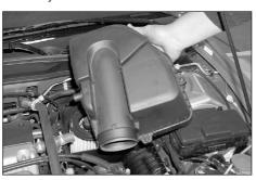
7. Loosen the five bolts that secure the upper air cleaner assembly, then remove the assembly as shown.
