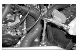
10. Loosen and remove the hex bolt that secures the air inlet duct as shown.
