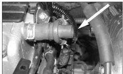
14. **On '05-'06** models, remove the stock crankcase vent hose as shown.
