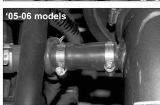
18. Connect the crank case vent hose to the vent on the K&N intake tube and slide the stock hose clamp onto the vent as shown. On 2005-06 model, use supplied hose and hose clamps and tighten.
