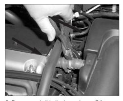
3. Depress and slide the hose clamp off the crank case vent connection at the air cleaner assembly as shown.
