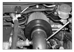
23. Install the K&N Filtercharger onto the K&N intake tube, then, secure with the provided hose clamp as shown.
