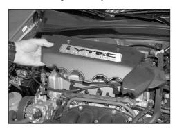
Loosen and remove the two bolts that secure the engine cover, then remove the engine cover as shown.
