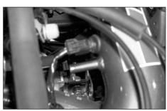
21. Push the air temperature sensor into the grommet in the K&N intake tube as shown.
