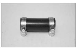
15. **On '05-'06 models,** place hose clamps on each side on 08692 Silicone Hose, as shown.
