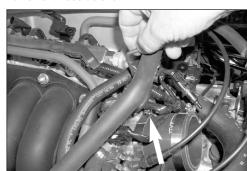
13. Install the silicone hose and hose clamps onto the throttle body and tighten as shown. NOTE: On 2002-04 model years, advance to step #16.
