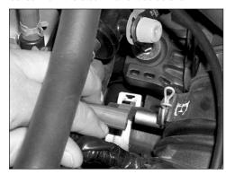
5. Disconnect the IA bypass control thermal valve vent hose from the stock intake tube as shown.
