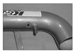
16. Install the provided grommet into the hole on the K&N intake tube as shown.
