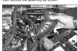
9. Loosen the hose clamp at the throttle body, then remove the stock intake tube as shown.
