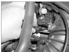
4. Depress the hose clamp at the air temperature sensor, then remove the air temperature sensor from the stock intake tube as shown.
