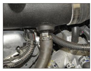
31. Connect the crank case vent hose to the fitting installed into the K&N® intake tube and secure with the factory hose clamp.
