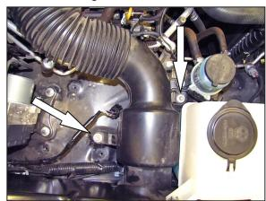
6. Remove the two bolts securing the intake resonator to the inner fender and then remove the intake tube/resonator assembly from the engine compartment.
