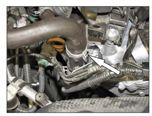
3. Release the spring clamp securing the secondary air hose to the union on the engine and then disconnect the secondary air hose.
