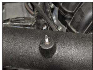
35. Install the engine cover mounting stud into the  $K\&N^{\scriptsize @}$  intake tube.
