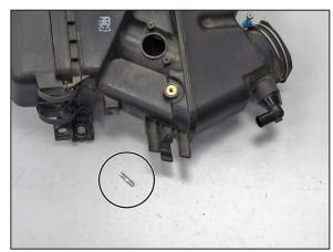
34. Remove the engine cover mounting stud from the factory air filter housing.
