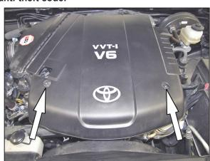
2. Remove the two nuts which secure the engine cover and then lift off the engine cover.
