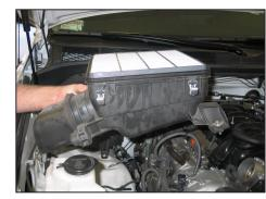
7. Loosen the two bolts securing the lower air box and then remove the lower air box from the vehicle. **NOTE: K&N Engineering, Inc., recommends that customers do not discard factory air intake.**
