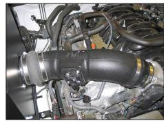
24. Insert the K&N<sup>®</sup> intake tube into the hump hose attached to the heat shield and then into the step hose attached to the throttle body. Secure with the provided hose clamps.
