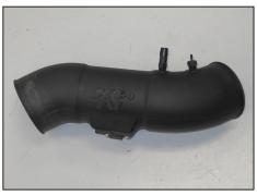
21. Install the provided NPT vent fittings into the K&N $^{\circ}$  intake tube as shown.
