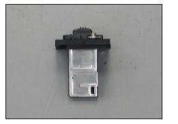
19. Install the mass air sensor through the K&N®
