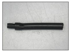
22. Install the hose mender into the provided crank case vent hose as shown.
