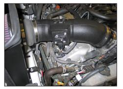
27. Reconnect the mass air sensor electrical connection.
