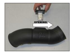
20. Install the mass air sensor assembly into the  $K\&N^{\oplus}$  intake tube so that the opening in the sensor faces the filter end of the tube as shown.
