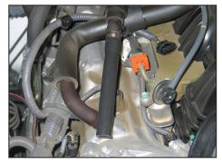
23. Install the crank case vent hose assembly into the factory crank case vent hose as shown.
