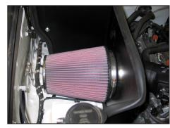
26. Install the K&N<sup>®</sup> air filter and secure with the provided hose clamp. NOTE: Drycharger<sup>®</sup> air filter wrap; part # RF-1020DK is available to purchase separately. To learn more about Drycharger<sup>®</sup> filter wraps or look up color availability please visit http://www.knfilters.com<sup>®</sup>.
