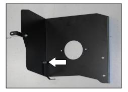
10. Install the heat shield mounting bracket (07190) onto the heat shield using the provided spacer and hardware.
