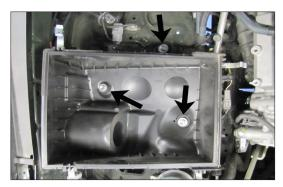
9. Loosen and remove the three bolts securing the lower air box and then remove the lower air box from the vehicle.
