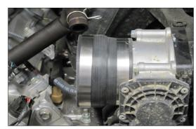
21. Install the provided silicone step hose (084091) onto the throttle body and secure with the provided hose clamp.
