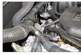
4. Unhook the fuel pressure vent line from the fuel pressure regulator.
