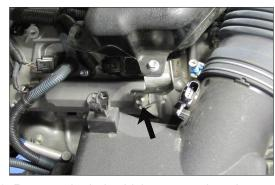
6. Remove the bolt which secures the tube mounting bracket to the engine valve cover.
