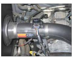
34. Reconnect the Mass air sensor electrical connection.
