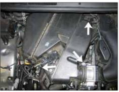
7. Loosen the hose clamp at the throttle body and then remove the two air box mounting bolts shown. 9. Install the "L" bracket (070742) onto the heat shield as shown using the provided hardware.
