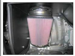
32. Install the filter assembly onto the K&N<sup>®</sup> Intake Tube and secure with the provided hose clamp.
