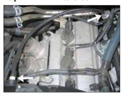
33. Install the provided vacuum hose onto the fuel pressure regulator and then attach the open end to the  $\frac{1}{4}$ "npt fitting installed into the K&N<sup>®</sup> Intake Tube.
