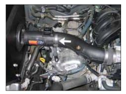
28. Install the K&N<sup>®</sup> Intake Tube assembly into the silicone hose at the throttle body and align with the tube mounting bracket assembly, then secure with the provided hose clamps.
