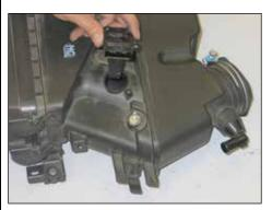
23. Remove the mass air sensor from the stock air box as shown.
