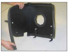
13. Install the provided edge trim around the heat shield as shown.NOTE: Some trimming of the edge trim will be necessary.
