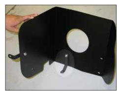
10. Install the "L" bracket (07190) onto the heat shield as shown using the provided hardware.
