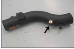
27. Install the provided rubber mounted stud onto the K&N<sup>®</sup> Intake Tube as shown.
