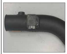
25. Install the mass air sensor into the K&N<sup>®</sup> Intake Tube and secure with the provided bolts and spacers.
