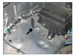
12. Install the "L" bracket (070089) onto the inner fender as shown.NOTE: The bolt will thread into the threaded hole in the inner fender.
