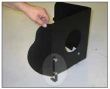
11. Install the "L" bracket (070902) onto the heat shield as shown using the provided hardware.
