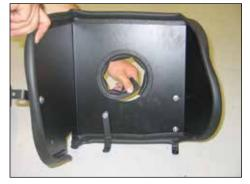
14. Install the provided edge trim inside the opening as shown.NOTE: Some trimming of the edge trim
