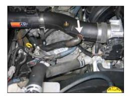
29. Reconnect the crank case vent hose to the K&N $^{\circ}$  Intake Tube as shown.
