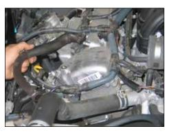
19. Remove the crank case vent hose from the valve cover.
