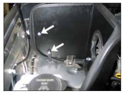
17. Secure the rear of the heat shield to the bracket installed in step #12 using the hardware and spacer provided. Secure the heat shield to the upper bracket with the hardware provided.
