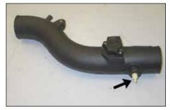
26. Install the ¼"npt fitting into the K&N<sup>®</sup> Intake Tube as shown.
