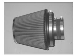
27. Install the silicone hose (08630) onto the filter adapter as shown and secure with the provided hose clamp.
