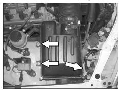
6. Loosen the three bolts that secure the stock airbox assembly to the inner fender.
