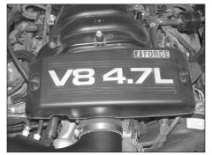
29. Reinstall the engine cover and secure with the nuts removed in step #3.
