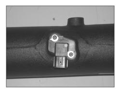
10. Install the mass air sensor into the K&N<sup>®</sup> intake tube and secure with the provided spacers and hardware as shown.
