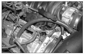
23. Install the provided crankcase vent hose onto the valve cover and then attach to the intake tube as shown.
