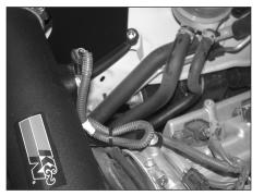
31. Using the provided wire tie, safely secure the excess mass air sensor wiring.
