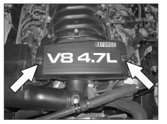
3. Loosen and remove the nuts shown that secure the throttle body cover, then remove the throttle body cover from the engine.
