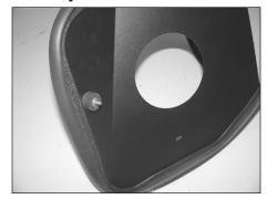
12. Install the rubber mounted studs onto the heat shield as shown using the provided hardware.
