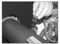
30. Reconnect the mass air sensor electrical connection as shown.
