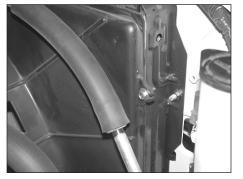
15. Remove the radiator fan shroud upper mounting bolt shown. **NOTE: This bolt will be reused.**
