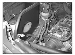
17a. Install the tube mounting bracket (083113) onto the heat shield a shown using the provided hardware.
