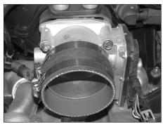
18. Install the silicone hose (08630) onto the throttle body and secure with the provided hose clamp as shown.
