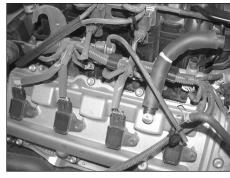
22. Remove the factory crankcase vent hose and fuel pressure regulator vent hose shown from the engine.
