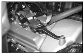
19. Install the tube mounting bracket assembly onto the valve cover with the provided hardware as shown.
