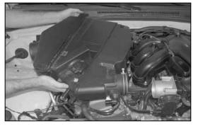
11. Remove the air box assembly from the engine as shown.
