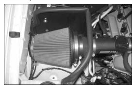
32. Install the K&N<sup>®</sup> air filter onto the intake tube as shown.
