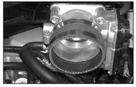
20. Install the silicone hose (08434) onto the throttle body with the provided hose clamps as shown.
