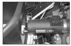
27. Secure the K&N<sup>®</sup> intake tube to the saddle bracket with the provided hose clamps. Also tighten the hose clamp attached to the throttle body.
