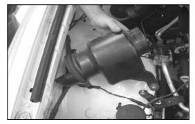
6. Remove the two bolts that secure the resonator to the inner fender, then remove the resonator from the vehicle as shown.
