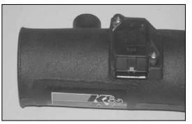
23. Secure the mass air sensor to the K&N<sup>®</sup> intake tube using the provided screws and spacers as shown
