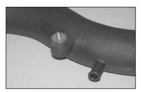
25. Install the rubber mounted stud onto the K&N<sup>®</sup> intake tube as shown.
