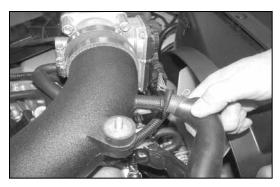
29. Install the original crank case vent hose onto the valve cover, then connect the opposite end of the crank case vent hose onto the K&N<sup>®</sup> intake tube.
