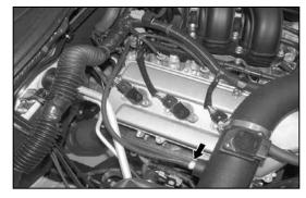
28. Remove the stock vacuum hose from fuel pressure regulator. Attach the provided silicone hose to the fuel pressure regulator and then onto the K&N<sup>®</sup> intake tube.
