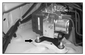
15. Remove the ABS pump mounting nut shown. NOTE: This nut will be reused. Some vehicles may not be equipped with the ABS pump.
