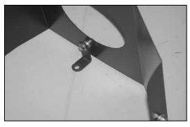
13. Install the small heat shield mounting bracket (070812) with the provided spacer onto the heat shield as shown.
