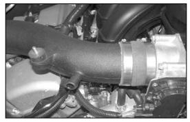
26. Install the K&N<sup>®</sup> intake tube onto the throttle body and align with the saddle bracket.
