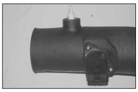
24. Install the vent fitting into the K&N<sup>®</sup> intake tube as shown.
