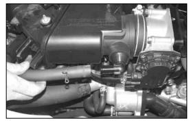
8. Remove the crank case vent hose from the air box as shown.
