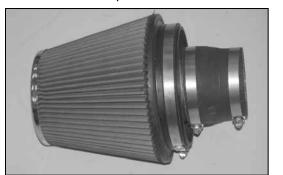
31. Install the provided silicone hose (08724) onto the air filter assembly and secure with the provided hose clamp as shown.
