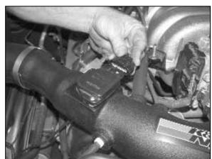
25. Reconnect the mass air sensor electrical connections.
