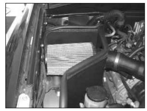
22. Install the K&N® air filter onto the intake tube as shown.
