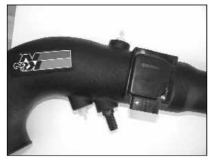
18. Assemble the vent fittings onto the K&N® intake tube as shown.
