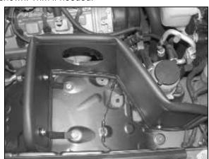
11. Install the heat shield onto the vehicle then secure to brackets with the provided hardware.
