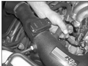
21. Install the provided silicone hose onto the K&N® intake tube and re-connect the one existing vent line as shown.
