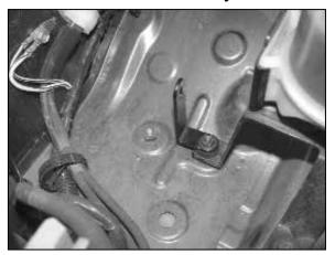
8. Remove the 12mm bolt that retains the power steering reserve to vehicle then mount the provided bracket (070632) onto the vehicle with the bolt that was removed.
