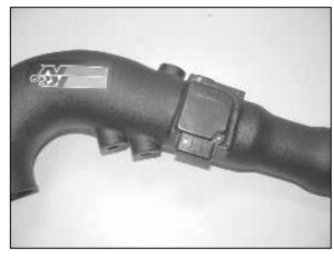
17. Secure the mass air sensor to the K&N® intake tube using the provided screws and spacers as shown.
