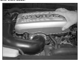
2. Loosen the two nuts that secure the throttle body cover then remove the throttle body cover.
