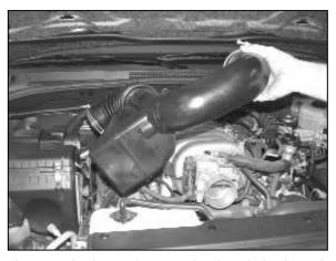
5. Loosen the hose clamp at the throttle body and air box, then remove intake tube from vehicle.
