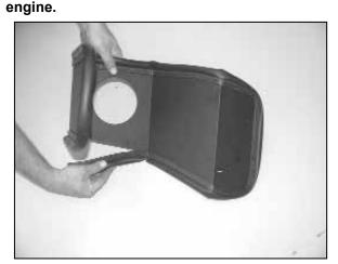
10. Install the edge trim onto the heat shield as shown. Trim if needed.
