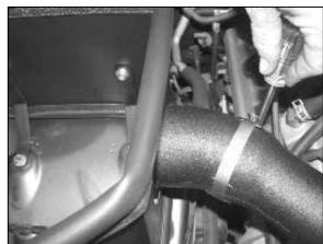
20. Secure the K&N® intake tube to the saddle bracket with the provided hose clamps also tighten the hose clamp at the throttle body.
