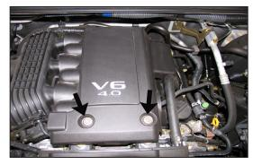
3. Remove the two bolts shown, which secure the engine cover.
