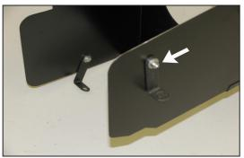
14. Install the "L" bracket (07805) onto the heat shield as shown with the provided hardware.
