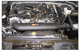
23. Install the K&N® intake tube into the silicone hose at the throttle body and align with the tube mounting bracket installed in step #16. Secure with the provided hardware and hose clamp.
