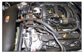
24. Attach the provided silicone crank case vent hose to the valve cover and K&N® intake tube as shown.
