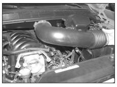
5. Loosen the hose clamps at the throttle body and air box, then remove the intake tube from the vehicle.
