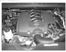
32. Re-install the throttle body cover as shown.
