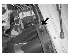
7. Remove the air box mounting bolt with a 10mm socket.
