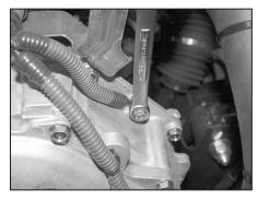
16. Locate the ground wire attached to the engine cam cover and remove the bolt securing it using a 10mm wrench.
