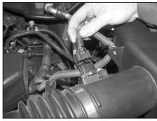
3. Disconnect the mass air sensor electrical connection, then release the wire loom from the air box
