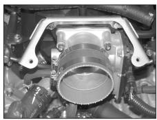
18. Install the provided silicone hose (08690) onto the throttle body with the provided hose clamps as shown.
