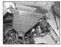
8. Pull firmly up on the air box to release it from the mounting studs, then remove the air box from the vehicle.
