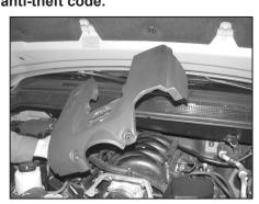
2. Remove the two bolts that secure the throttle body cover, then remove the throttle body cover.
