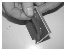
20. Apply the provided gasket to the mass air sensor adapter as shown; sticky side down.
