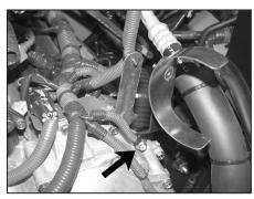
17. Install the saddle bracket assembly and ground wire removed in step #16 with the provided hardware as shown.
