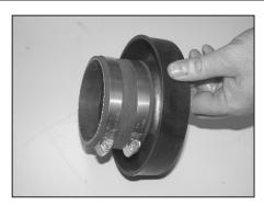
28. Install the provided silicone hose (#08630) onto the filter adapter as shown.
