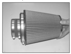
29. Install the filter adapter assembly into the K&N® air filter.
