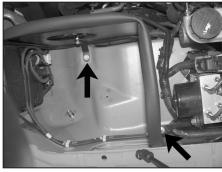
14. Install the heat shield onto the vehicle and secure with the provided hardware.
