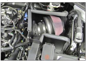
20. Install the provided step coupler (08496) onto the filter adapter and secure with the provided hose clamp.
