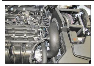
23. Install the K&N® intake tube into the coupling hose at the filter adapter and then into the hose at the throttle body, adjust the tube for best fit and then secure with the provided hose clamps.
