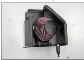
15. Install the K&N® air filter onto the filter adapter and secure with the provided hose clamp.
