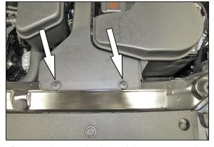
3. Remove the two plastic retaining screws and then remove the fresh air intake duct from the vehicle.
