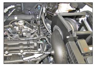
24. Connect the factory crank case vent hose to the fitting installed into the K&N® intake tube and then connect the EVAP hose to the factory valve.
