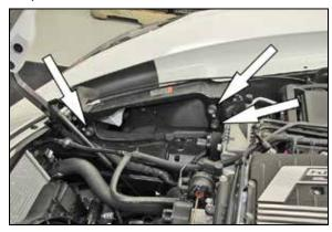
15. Install the three provided rubber mounted studs onto the air filter housing mounting locations as shown. 20. Install the provided coupling hose (08761) onto the throttle body and secure with the provided hose clamp.
