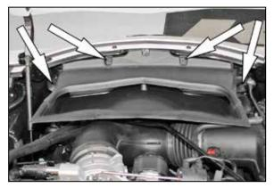
2. Remove the four bolts that secure the air extraction duct to the radiator and then remove the air extraction duct from the vehicle.
