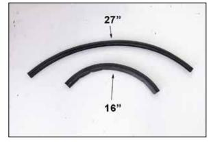
16. Cut the provided edge trim into two sections, one section will be 27" long and the other section will be 16" long.
