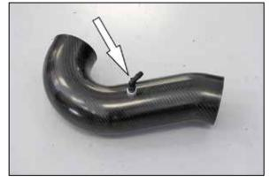
23. Install the provided 90° npt fitting into the K&N $^{\odot}$  intake tube as shown.
