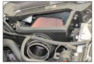
19. Install the heat shield/filter assembly onto the rubber mounted studs installed during step #13 and secure with the provided hardware.
