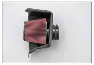
18. Set the air filter into the heat shield and then install the coupling hose (08761) onto the filter and secure with the provided hose clamp.
