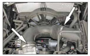
5. Loosen the two hose clamps that secure the factory intake tube to the throttle body and to the air filter housing and then remove the factory intake tube from the vehicle.
