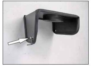
12. Install the heat shield mounting bracket (070812) onto the heat shield using the provided hardware and spacer.
