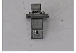
20. Install the factory mass air sensor into the K&N<sup>®</sup> adapter assemble and secure with the provided hardware.
