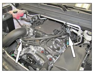
25. Install the crank case vent hose onto the fitting installed into the K&N<sup>®</sup> intake tube and then connect the hose mender into the fitting on the valve cover.
