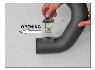
21. Install the mass air sensor assembly into the K&N<sup>®</sup> intake tube and secure with the provided hardware.
