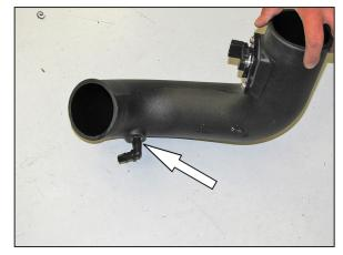
22. Install the provided 90° vent fitting into the K&N $^{\circ}$  intake tube as shown.
