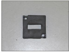
18. Install the provided gasket onto the K&N $^{\mbox{\tiny \$}}$  mass air sensor adapter.
