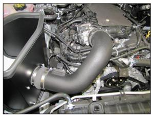
23. Install the K&N<sup>®</sup> intake tube into the hump coupler and then into the step coupler at the throttle body, adjust the tube for best fit and then secure with the provided hose clamps.
