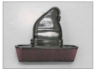
9. Install the two hose clamps onto the silicone hose and secure the filter to the intake tube with the clamps.
