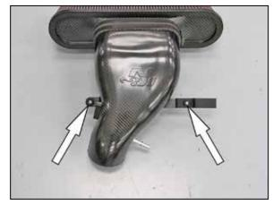
12. Install the factory mounting grommets into the  $K\&N^{\otimes}$  mounting bracket as shown.
