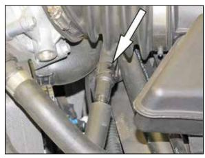
4. Disconnect the crank case vent tube from intake tube.
