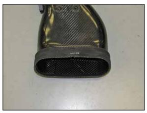
7. Slide the silicone hose (08619) onto the K&N<sup> $\otimes$ </sup> intake tube so that only approximately <sup>1</sup>/<sub>4</sub>" of the hose is not installed.
