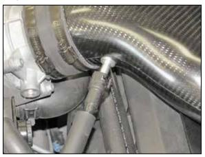
16. Connect the crank case vent tube to the fitting on the  $K\&N^{\otimes}$  intake tube.
