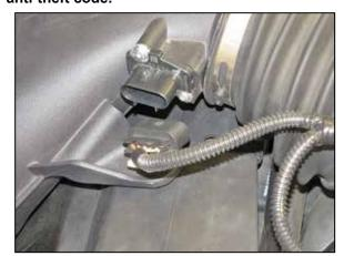
Disconnect the mass air sensor electrica
