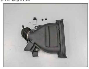
11. Remove the two bolts securing the mass air sensor into the factory intake tube and then remove the mass air sensor. Remove the two factory rubber mounting grommets from the factory intake.
