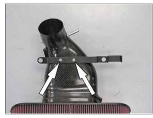
10. Install the tube mounting bracket onto the K&N<sup>®</sup> intake tube using the provided hardware. NOTE: Be sure to place the two rubber washers between the bracket and intake tube. Be sure to apply the provided thread locker to the bracket mounting bolts.
