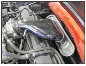
15. Install the K&N<sup>®</sup> intake system onto the mounting studs, then slide the silicone hose onto the throttle body and secure with the provided hose clamps.
