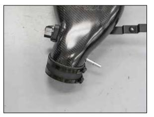
14. Install the provided silicone hose (08761) onto the K&N $^{\circ}$  intake tube but do not tighten the hose clamps at this time.
