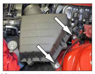
5. Remove the two air box mounting nuts shown.
