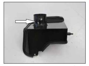
12. Install the mass air sensor into the K&N® mass air sensor housing and secure with the provided hardware.
