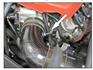
19. Install the provided crank case vent fitting into grommet in the K&N® intake tube as shown.
