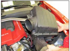
6. Remove the air box from the vehicle.
