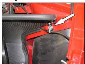
14. Secure the heat shield using the factory air box mounting nut and then install the ground cable mounting lug onto the stud.
