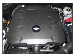
2. Remove the oil fill cap, lift up and remove the engine cover. Reinstall the oil cap.
