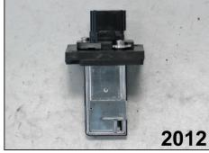
18. Install the mass air sensor into the mass air sensor adapter and secure with the provided hardware.
