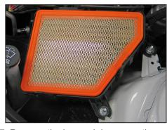
7. Remove the lower air box mounting nuts, then remove the lower air box assembly.
