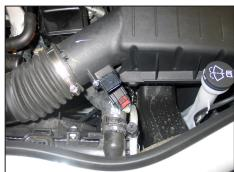
3. Slide the red locking tab back and then disconnect the mass air sensor electrical connection.
