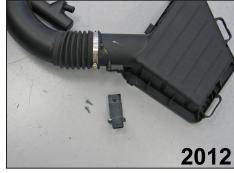
17. Remove the two screws that secure the mass air sensor into the factory intake tube.
