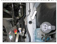
8. Remove the air box mounting grommet shown on the frame rail.
