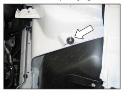
13. Install the provided rubber fender washer onto the outer air box mounting stud.
