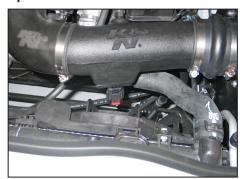
24. Reconnect the mass air sensor electrical connection.
