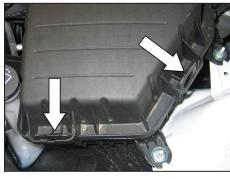
6. Unlatch the upper air box clips and remove the upper air box and intake tube assembly.
