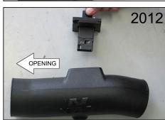
19. Install the mass air sensor assembly into the  $K\&N^{\otimes}$  intake tube as shown and secure with the provided hardware.
