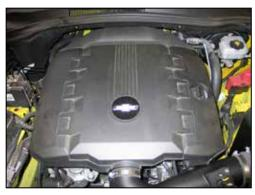
26. Reinstall the engine cover and secure with the oil fill cap.
