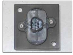
20. Install the mass air sensor into the K&N® mass air sensor adapter and secure with the provided hardware.
