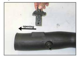
21. Install the mass air sensor assembly into the K&N® intake tube so that the opening faces toward the filter end of the tube; secure with the provided hardware.
