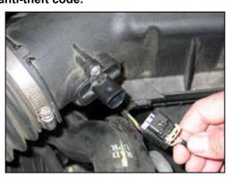
2. Release the locking and then disconnect the mass air sensor electrical connector.
