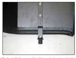
12. Install the provided inserted nut onto the heat shield mounting bracket and secure with the provided hardware.
