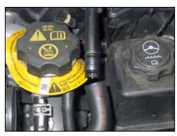
4. Disconnect the crank case vent hard line from the 90°connector hose on the factory intake tube.
