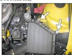
6. Remove the two nuts shown securing the factory air box to the inner fender.
