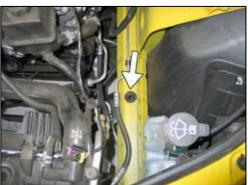
8. Remove the air box mounting grommet shown from the inner fender.
