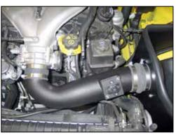
22. Install the K&N® intake tube into the silicone hump hose and then into the silicone hose at the throttle body and secure with the provided hose clamps.
