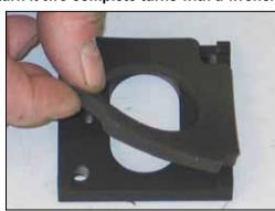
18. Peal the backing paper off and then install the provided gasket onto the K&N® mass air sensor adapter as shown.
