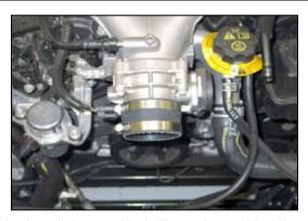
15. Install the provided silicone hose (08711) onto the throttle body and secure with the provided hose clamp.
