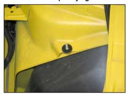
13. Install the provided rubber fender washer onto the outward air box mounting stud.
