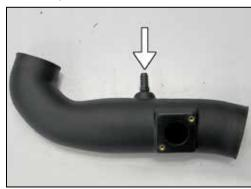
17. Install the provided 1/4 NPT vent fitting into the K&N® intake tube as shown.
