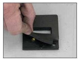
19. Install the provided gasket onto the mass air sensor adapter as shown.
