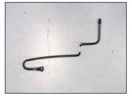
24a. On 2014 and later vehicles, it will be necessary to cut the crank case vent tube as shown. Then connect the cut section of tube to the oil filler cap. Attach the supplied hose to the to the trimmed section of crank case vent tube,
