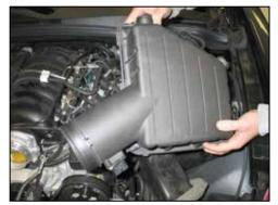
9. Lift up and remove the air box from the vehicle. NOTE: K&N Engineering, Inc., recommends that customers do not discard factory air intake.
