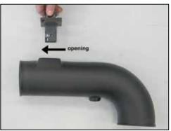
21. Install the mass air sensor assembly into the K&N^ $\ensuremath{\mathbb{R}}$  intake tube and secure with the provided hardware.
