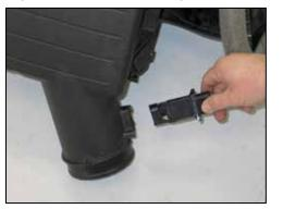
18. Remove the two screws and then remove the mass air sensor from the factory air box.
