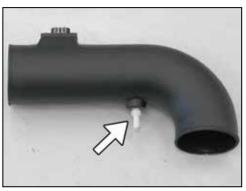
22. Install the provided 1/4 NPT fitting into the K&N^ $\ensuremath{\mathbb{R}}$  intake tube as shown.
