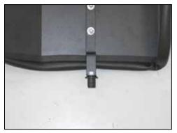
14. Install the inserted nut onto the heat shield mounting bracket using the provided hardware. Do not completely tighten at this time.
