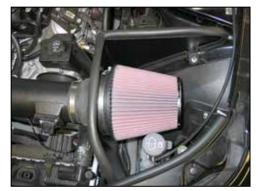
25. Install the K&N<sup>®</sup> air filter onto the filter adapter and secure with the provided hose clamp. NOTE: Drycharger<sup>®</sup> air filter wrap; part # RF-1042DK is available to purchase separately. To learn more about Drycharger<sup>®</sup> filter wraps or look up color availability please visit http://www.knfilters.com<sup>®</sup>.
