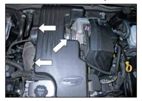
6. Loosen the two intake resonator mounting bolts and hose clamp at the throttle body. **NOTE: One intake resonator mounting bolt will be re-used.**
