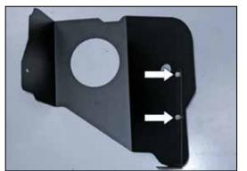
9. Install "L" bracket (#010060) onto the heat shield with the provided hardware as shown. **NOTE: Use two of the provided spacers between the bracket and heat shield, one on each bolt.**
