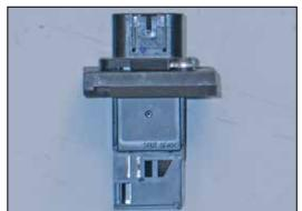
15. Install the mass air sensor into the K&N<sup>®</sup> mass air sensor adapter and secure with the provided hardware as shown.
