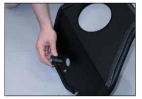
11c. Install the provided adapter into the small heat shield hole as shown.
