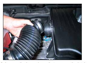
3. Loosen the hose clamp that secures the intake tube to the intake resonator. Disconnect the intake tube from the intake resonator as shown.
