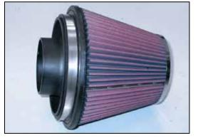
22. Install the provided air filter adapter into the K&N<sup>®</sup> air filter and secure with the provided hose clamp.
