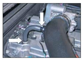
21. Install the provided crank case vent hose onto the valve cover and connect the remaining open end to the K&N<sup>®</sup> intake tube as shown. NOTE: Some trimming of the provided crank case vent hose may be necessary.
