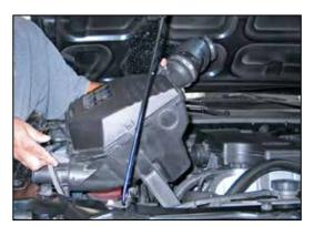
5. Lift the air box up, removing it from the vehicle. **NOTE: K&N Engineering, Inc., recommends that** customers do not discard factory air intake
