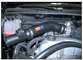
20. Install the K&N<sup>®</sup> intake tube into the silicone hose at the throttle body and align it with the mounting bracket installed in the previous step. Secure the intake tube with the provided hose clamps.
