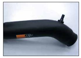
17. Install the provided  $\frac{1}{4}$ " NPT fitting into the K&N<sup>®</sup> intake tube as shown.
