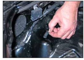
11b. Install the provided insert nut into the hole drilled into the fender in step #11a.
