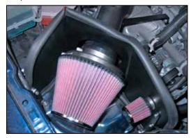
24. Install the air filter assembly onto the K&N<sup>®</sup> intake tube and secure with the provided hose clamp.
