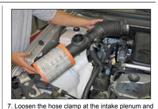
then remove the complete intake system. NOTE: K&N Engineering, Inc., recommends that
