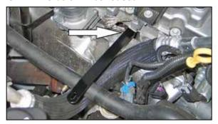
12. Install the tube mounting bracket (26632) onto the engine at the ground cable location and secure with the bolt removed in step #11.
