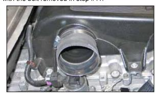
13. Install the provided silicone hose (08051) to the throttle body and secure it with the provided hose clamp.
