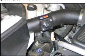
19. Cut the air injection hose at the location marked in step #18. Then install the hose onto the K&N® intake tube and secure with the provided hose clamp.
