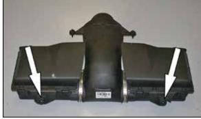
5. Remove the two rubber mounting grommets shown air box as shown.
