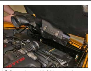
4. Pull up on the complete intake system to disconnect it from the air box mounting pins and then remove it from the vehicle as shown.
