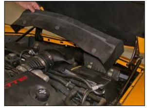
2. Unsnap the ends and then remove the air filter cover as shown.
