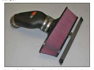
10. Install the air filter mounting bracket onto the air filter as shown and secure with the provided hardware.
