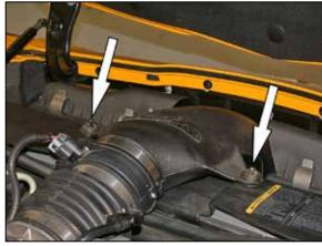
3. Loosen the hose clamp which secures the stock intake tube to the mass air sensor, then pull up to release the center locking pins in the intake tube mounting fasteners shown.
