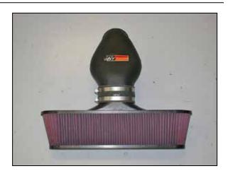
8. Install the K&N® intake tube onto the air filter as shown and secure with the provided hose clamp.
