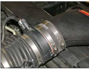
13. Install the intake kit onto the mass air sensor secure with the provided hose clamp.
