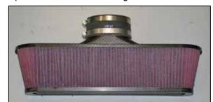
7. Install the silicone hose (08625) onto the air filter as shown and secure with the provided hose clamps
