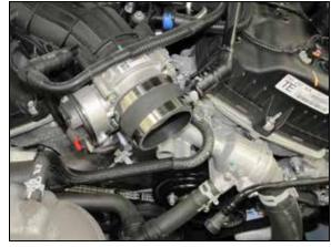
12. Install the provided straight coupler (08711) onto the throttle body and secure with the provided hose clamp.
