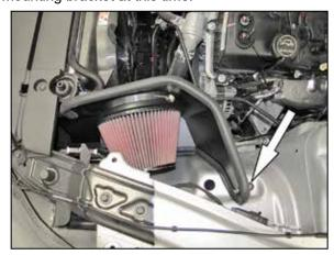
10. Flex the heat shield back and install the K&N® air filter onto the adapter then secure the filter with the hose clamp. Secure the upper heat shield mounting bracket with the hardware provided. NOTE: Drycharger® air filter wrap; part # 22-8049DK is available to purchase separately. To learn more about Drycharger® filter wraps or look up color availability please visit http://www.knfilters.com®.
