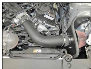
14. Install the intake tube fully into the hump coupler and then into the straight coupler at the throttle body, adjust the tube for best fit and then secure with the provide hose clamps.
