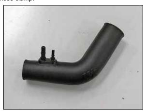
13. Install Quick disconnect fittings into the K&N® intake tube as shown.
