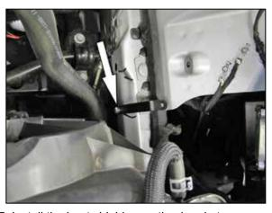
5. Install the heat shield mounting bracket (064325) onto the inner frame rail with the provided hardware as shown.
