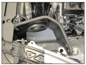
9. Install the heat shield onto the lower mounting bracket and then secure it only to the lower mounting bracket at this time.
