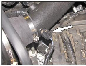
23. Connect the inlet air temperature sensor electrical connection.
