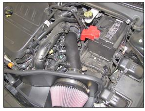
21. Install the K&N® intake tube assembly into the coupling hose at the turbo inlet and then into the coupling hose at the filter adapter. Adjust the tube for best fit and then secure with the provided clamps.
