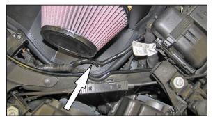
16. Clip the inlet air temperature sensor harness into the hole provided in the heat shield.
