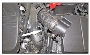
3. Disconnect the crank case vent hose from the factory intake tube.
