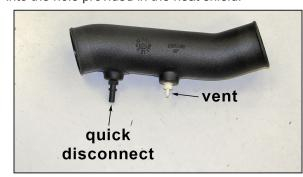
17. Install the provided 1/4"npt fittings into the K&N® intake tube as shown.
