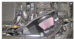
15. Set the heat shield assembly into the vehicle. The mounting stud will insert into the factory air box mounting grommet and the front of the heat shield will be secured to the core support with the provided hardware.
