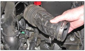
7. Loosen the hose clamp securing the factory intake tube to the turbo and then remove the hose from the vehicle.
