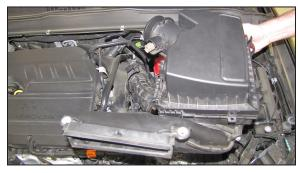
6. Lift up the air box to dislodge it from the mounting grommets and then remove it from the vehicle.
