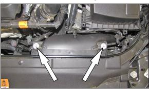
5. Remove the two bolts securing the fresh air intake scoop.
