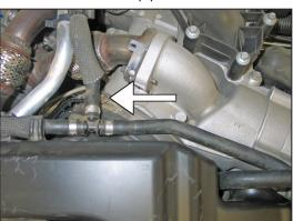
8. Loosen the hose clamp that secures the intake tube to the engine inlet.
