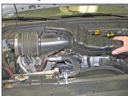
9. Remove the intake tube from the vehicle.
