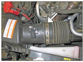
3. Loosen the hose clamp that secures the intake tube to the upper air box.
