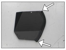
39. Install the provided edge trim onto the heat shield lid as shown.
