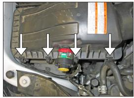
4. Release the four upper air box retaining clips.
