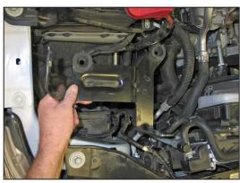
13. Remove the air box mounting bracket from the vehicle.
