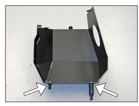
20. Install the two heat shield stand-offs onto the heat shield as shown using the provided hardware.
