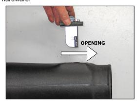
29. Install the mass air sensor assembly into the  $K\&N^{\scriptsize @}$  intake tube as shown and secure with the provided hardware.
