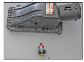
36. Remove the filter minder from the factory upper air box.
