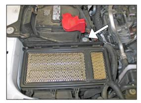
10. Remove the bolt securing the lower air box to the battery tray.
