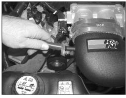
20. Install the supplied vent hose onto the vent port on the valve cover and then onto the K&N® intake tube as shown.
