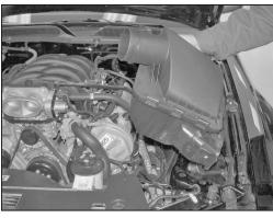
6. Remove the air box assembly as shown.
