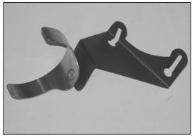
7. Install the saddle clamp onto the tubemounting bracket as shown with the provided hardware.
