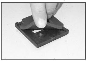
17. Install the provided gasket to the back of the  $K\&N^{\otimes}$  mass air sensor adaptor plate as shown.
