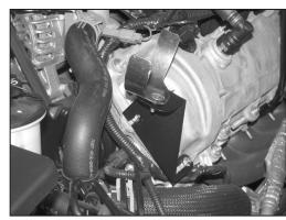
10. Install the tube-mounting bracket onto the valve cover as shown and secure with the stock hardware removed in step #8.
