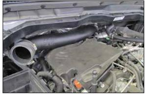
8. Install the K&N $^{\circ}$  intake tube into the factory turbo inlet hose and secure with the factory hose clamp.
