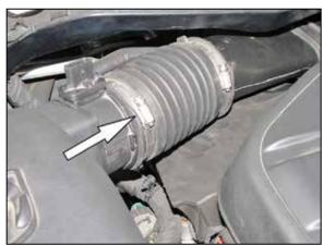
3. Loosen the hose clamp securing the factory intake tube to the mass air sensor.
