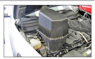
5. Lift up the air filter housing to dislodge it from the mounting grommets and then remove the complete air filter housing assembly from the vehicle.
