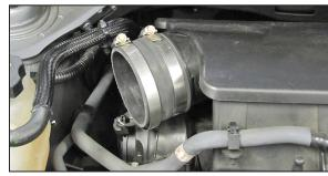
14. Install the provided coupler hose (08690) onto the intake plenum and secure with the provided hose clamp.
