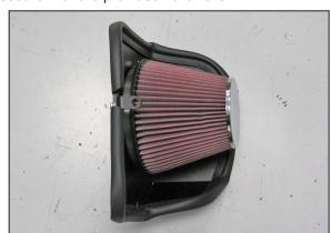
12. Install the K&N® air filter onto the filter adapter and secure with the provided hose clamp. NOTE: Drycharger® air filter wrap; part # RF-1048DK is available to purchase separately. To learn more about Drycharger® filter wraps or look up color availability please visit http://www.knfilters.com®.
