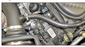
20. Install the factory quick disconnect fitting into the provided crank case vent hose and then install the assembly onto the factory hardline and connect the quick disconnect fitting to the fitting installed into the K&N® intake tube.
