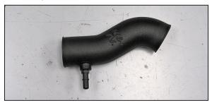
15. Install the provided quick disconnect fitting into the K&N® intake tube as shown.
