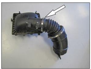
8. Loosen hose clamp securing intake resonator to air box lid and remove intake resonator from lid.
