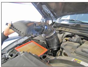
5. Remove air box lid and intake resonator from the vehicle.
