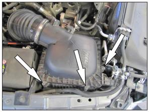
4. Remove the three screws securing air box lid.
