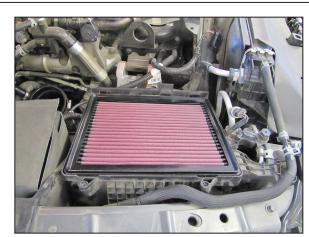
7. Install K&N® filter into air box base.
