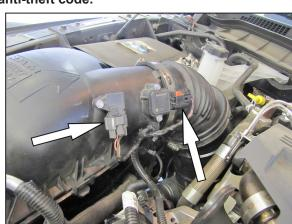
2. Disconnect mass air sensor and temperature sensor electrical connections, then unhook the wiring harness from air box.
