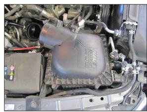
9. Reinstall air box lid onto air box base.
