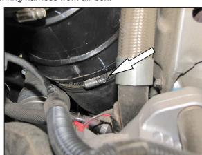
3. Loosen the hose clamp securing the intake resonator to turbo inlet hose.
