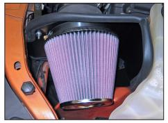
24. Install the K&N<sup>®</sup> air filter and secure with the provided hose clamp. NOTE: Drycharger<sup>®</sup> air filter wrap; part # RF-1042DK is available to purchase
