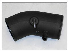
17. Install the provided  $90^{\circ}$  vent fitting into the K&N<sup>®</sup> intake tube as shown.
