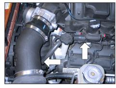
21. Install the assembled vent hose onto the fitting installed in the K&N<sup>®</sup> intake tube and then attach the open end to the valve cover port.
