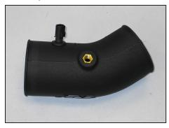
16. Install the provided grommet and the factory inlet air temperature sensor into the K&N<sup>®</sup> intake tube as shown.
