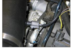
24. Connect the inlet air temperature sensor extension harness into the factory electrical connection and then connect the other end into the inlet air temperature sensor as shown.
