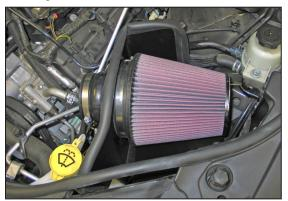
16. Install the K&N<sup>®</sup> filter onto the adapter and secure with the provided hose clamp. NOTE: Drycharger<sup>®</sup> air filter wrap; part # RF-1041DK is available to purchase separately. To learn more about Drycharger<sup>®</sup> filter wraps or look up color availability please visit http://www.knfilters.com<sup>®</sup>.
