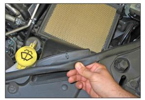
2. Lift up the engine cover to dislodge it from the mounting grommets and remove it from the vehicle.
