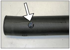
20. Install the inlet air temperature sensor into the  $K\&N^{\ensuremath{\mathbb{R}}}$  intake tube.
