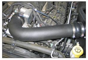
21. Install the K&N<sup>®</sup> intake tube into the hump hose at the filter adapter and then into the hose at the throttle body. Adjust the tube and heat shield for best fit and clearance and then secure with the provided hose clamps
