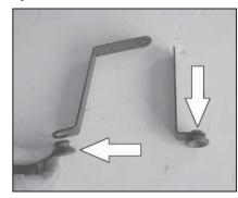
8. Install the two rubber bushings that were removed in the previous step into the provided brackets as shown.
