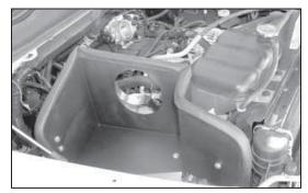
19. Install the heat shield onto the factory airbox studs then mount to the previously installed brackets.
