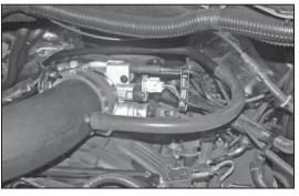
32. Connect the modified crankcase vent hose to the  $K\&N^{\otimes}$  intake tube as shown.
