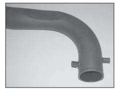
27. Install the air temp sensor into the  $K\&N^{\ensuremath{\circledast}}$  intake tube as shown.
