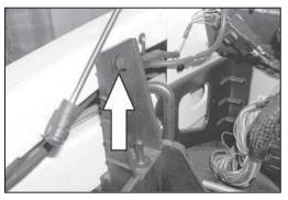
15. Remove the 8mm bolt that retains the airbox mount.
