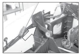
16. Install the twisted "L" bracket with the bolt that was removed in step 18. Do not tighten bolt completely.
