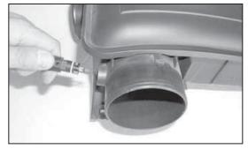
22. On models that come equipped with temp sensors, remove the air temp sensor from the resonator box as shown.
