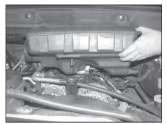
5. Pull up firmly to release the resonator from the engine.
