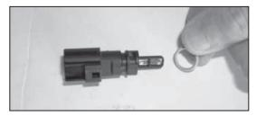
26. Remove the O-ring from the air temp. sensor as shown.
