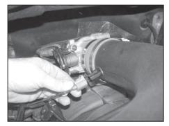
30. On models equipped with a air temp sensor, reconnect the electrical connection as shown. **NOTE:** Due to manufacturing tolerances, it may be necessary to use the provided extension harness to connect the inlet air temperature sensor electrical connection.
