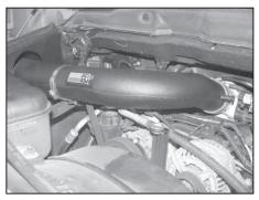
21. Install the intake tube onto the throttle body and saddle clamp and secure with the provided hose clamps as shown.
