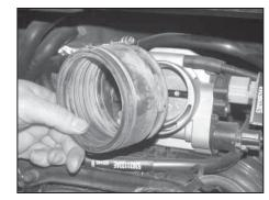
6. Loosen hose clamp that retains the rubber hose to the throttle body, then remove as shown.
