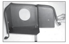
12. Install the provided edge trim onto the heat shield.
