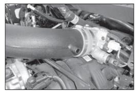
28. Install the intake tube onto the throttle body with the provided hose clamp.
