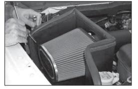
34. Align the heat shield for best clearance then tighten all the brackets.
