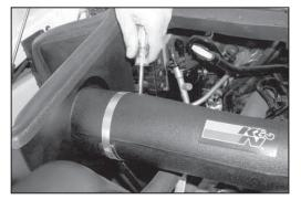
29. Using the provided hose clamp, secure the  $K\&N^{\ensuremath{\circledast}}$  intake tube to the saddle bracket assembly as shown.
