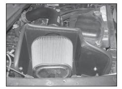
33. Install the K&N<sup>®</sup> air filter onto the K&N<sup>®</sup> intake tube as shown and secure with the hose clamp. **NOTE:** Drycharger<sup>®</sup> air filter wrap; part number **RF-1034DK** is available to purchase separately. To learn more about Drycharger<sup>®</sup> filter wraps or look up color availability please visit http:// www.knfilters.com<sup>®</sup>.
