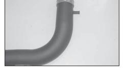
20.Install the provided silicone hose onto the  $K\&N^{\ensuremath{\circledast}}$  intake tube with the provided hose clamp as shown.
