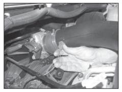
23. On vehicles equipped with an air temperature sensor, hold up the air temperature sensor wiring harness to the intake tube and mark the intake tube for drill point.
