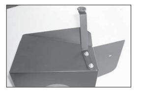
9. Install the large "Z" bracket onto the heat shield with the provided hardware. Do not tighten completely at this time.
