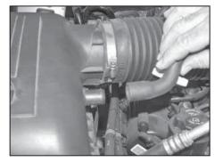
2a. On vehicles equipped, disconnect the crankcase vent from the airbox as shown. 4. Disconnect the inlet air temperature sensor electrical connection.
