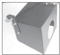
10. Install the "L" bracket onto the heat shield with the provided hardware. Do not tighten completely at this time.
