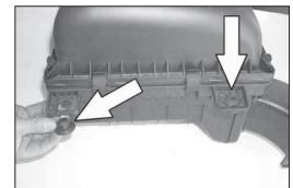
2. Loosen the hose clamp that connects the intake tube to the resonator box then remove the intake tube.
