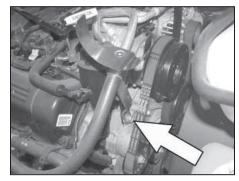
18. Install the saddle bracket assembly onto the belt tensioner using the provided spacer and hard-ware.
