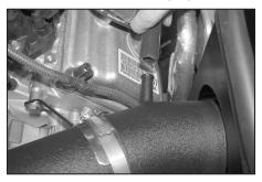
19. Install the provided crank case vent hose onto the vent port on the valve cover then install the vent hose onto the K&N<sup>®</sup> intake tube.
