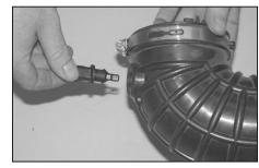
15. Remove the air temperature sensor from the factory intake tube.
