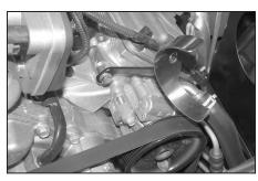
13. Using the provided spacer, install the tube mounting bracket assembly onto the engine as shown.
