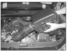
7. Lift the complete intake and air filter assembly to remove it from the vehicle.
