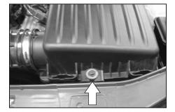
6. Loosen and remove the airbox mounting bolt as shown.
