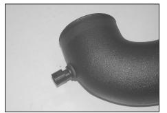
17. Install the factory air temperature sensor into the grommet installed in step #16.
