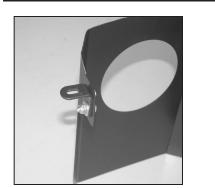
9. Install the "L" bracket (070066) onto the heat shield with the provided hardware through the non-slotted hole in the bracket.
