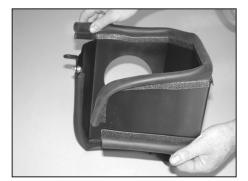
10. Install the two pieces of edge trim onto the heat shield as shown, be sure to leave a gap at the bracket mounting locations.
