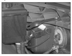
8. Install the twist bracket (070772) onto the core support using the hardware provided through the existing hole as shown.
