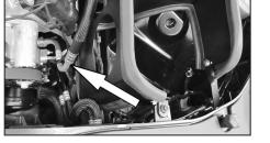
11a. Due to vehicle manufacturing tolerances, the A/C lines on some vehicles may need to repositioned slightly so that they do not contact the heat shield. To adjust, grab the A/C line on the aluminum section and carefully apply pressure in the desired direction until clearance is obtained.
