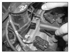
5. Disconnect the crank case vent hose from the valve cover port as shown.
