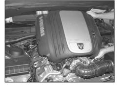
2. Lift up on the engine cover to loosen it from the mounts, and then remove the cover from the
