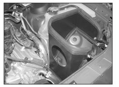
11. Install the heat shield assembly into the vehicle and secure to the bracket installed in step #8. Then secure the "L" bracket with the factory bolt removed in step #6 to the airbox mounting location.
