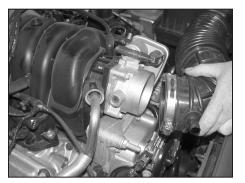
4. Loosen the hose clamp that secures the intake tube to the throttle body and pull the intake tube off of the throttle body.
