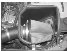
22. Install the air filter assembly onto the K&N<sup>®</sup> intake tube and secure with the provided hose clamp as shown.
