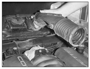
7. Detach the intake hose from the throttle body and remove the entire air intake assembly. **NOTE: K&N recommends that customers do not discard factory air intake.**
