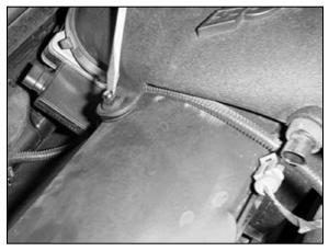
4. Release the push clips that retain the stock intake tube to the upper radiator cover.
