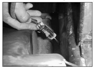
32. Detach the courtesy lamp wiring harness from the lower radiator cover and disconnect air temp. sensor at the right bottom corner of raidiator cover.
