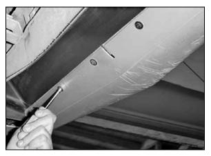
30. Loosen and remove the five bolts that mount the lower radiator cover to the bumper cover on the underside of the car.
