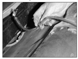
8. Detach the wiring harness retaining clip from the lower radiator cover.
