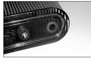
15. Install the 5/8" ID grommet and the rubber mounted stud into the top plate of the Air filter element.
