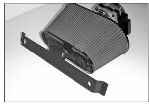
20. Attach the angled bracket to the rubber mounted stud using the provided hardware. **Note: Do not tighten completely at this time.**
