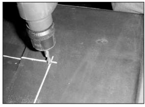
36. Using a 5/16" drill bit, drill a hole where the horizontal and vertical lines intersect.
