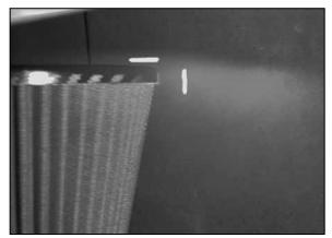
26. Using the Air filter element as a guide, mark a minimum of 1/2" away from the Air filter Element.
