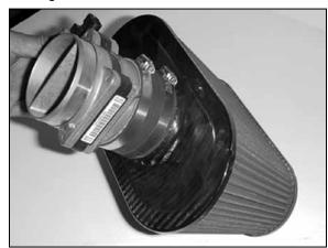
14. Install the mass air sensor into the silicone hose with the arrow on the mass air sensor pointing away from the Air filter element.
