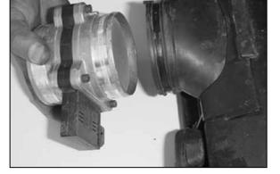
11. Remove the mass air sensor from the airbox.
