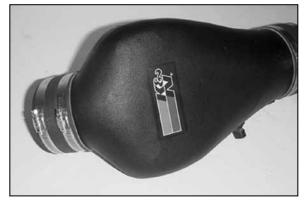
19. Install a 3.5" ID silicone hose (08630) onto the  $K\&N^{\circledast}$  intake tube.
