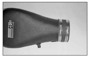
18. Install the 4" ID silicone hose (08755) onto the  $K\&N^{\circledast}$  intake tube.
