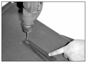
38. Hold the right angled "Z" bracket in place, using a 3/16" drill bit, drill out the five outer holes.
