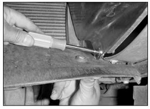
31. Loosen and remove the two bolts that retain the lower radiator cover to it's mounting brackets.
