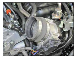
7. Install the provided coupling hose (08699) onto the throttle body and secure with the provided hose clamps as shown.
