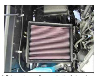
5. Release the two clips securing the factory air box lid and then remove the factory air filter. Install the provided  $K\&N^{\otimes}$  air filter into the air box, set the air box lid into position but do not secure at this time.
