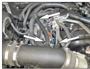
11. Install the crank case vent hose assembly into the factory crank case vent hose and then connect the open end to the fitting installed into the K&N® intake tube. Connect the factory fuel pressure regulator vent hose into the fitting installed into the K&N® intake tube.
