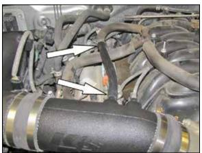
13. Install the union fitting into the K&N® crank case breather hose and then connect the hose to the factory crank case vent hose and the fitting installed into the K&N® intake tube.
