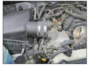
8. Install the provided coupling hose (08760) onto the air filter housing and secure with the provided hose clamp
