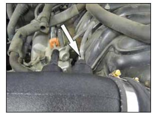
12. Connect the fuel pressure regulator vent hose to the fitting installed into the K&N® intake tube.
