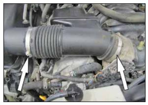
4. Loosen the two hose clamps securing the factory intake tube
