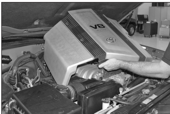
2. Remove the two bolts and two nuts that secure the engine cover, then remove the engine cover.
