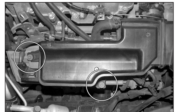
5. Remove the two bolts that secure resonator assembly to the motor.
