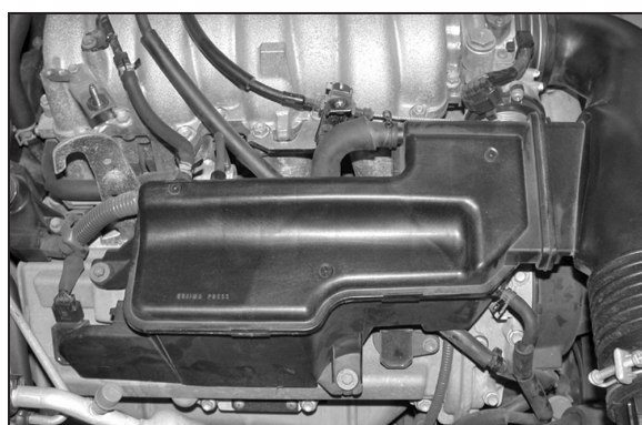
4. Remove the four vent lines from the air intake resonator as shown.
