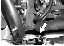
17. Secure the upper bracket to the fan shroud with the original bolt.
