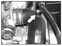
26. Re-connect the AC line to the K&N<sup>®</sup> intake tube using the original bolt.
