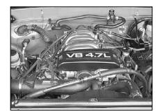
31. Re-install the throttle body cover onto the engine using the original acorn nuts.
