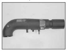
23a. Some 03 models, install the two vents and plug into the intake tube in the orientation as shown above.
