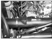
25. Secure the saddle bracket to the tube with the provided hose clamp.
