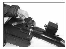
9. Loosen and remove the two screws that secure the mass-air sensor, then remove the mass air sensor.
