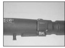
11. Install the mass-air sensor into the K&N<sup>®</sup> intake tube and secure with the provided spacers and screws as shown.
