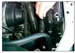
21. Using the hex bolt removed in step 17, secure the angled bracket to the radiator fan shroud as shown above. Do not tighten completely.
