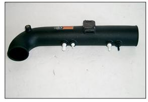
24. Assemble the vents onto the  $K\&N^{\ensuremath{\$}}$  intake tube as shown above.
