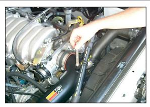
32. Using the hex bolt removed in step 5, secure the a/c hard line to the threaded boss on the K&N<sup>®</sup> intake tube.
