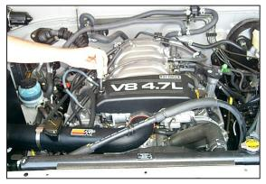
33. Re-install the throttle body cover as shown.
