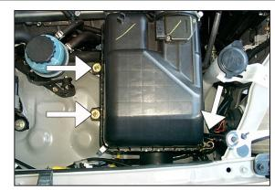
7. Loosen the three bolts that secure the air cleaner assembly to the inner fender.
