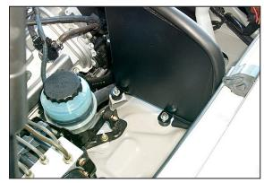
19. Secure the rear mounting tabs to the bumper studs with the provided hardware as shown.
