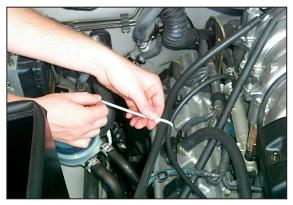
36. Zip tie the EVAP cannister vent hose and the fuel pressure regulator vent hose together as shown.
