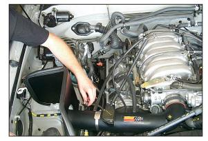
31. Install the three provided vent hoses onto the K&N $^{\circ}$  intake tube. Also re-connect the one existing vent as shown.
