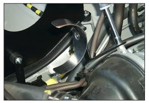
27. Install the saddle bracket assembly onto the threaded boss on the cam cover with the provided hardware as shown above.
