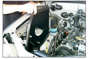
18. Install the heat shield assembly into the vehicle as shown.
