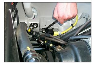
11. Remove the hex bolt from the inner fender as shown above.
