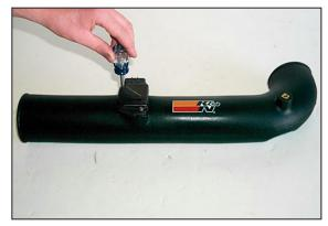
23. Secure the mass air sensor to the  $K\&N^{\otimes}$  intake tube using the provided spacers and screws.
