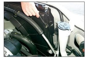
17. Remove the hex bolt from the radiator fan shroud as shown above.
