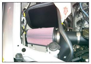
34. Install the K&N<sup>®</sup> air filter onto the K&N<sup>®</sup> intake tube as shown.
