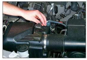
3. Disconnect the mass air sensor electrical connection.
