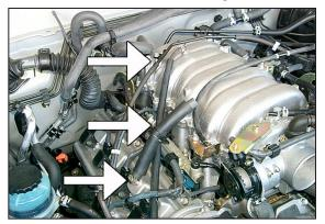
9. Remove the EVAP cannister vent hose, the crankcase vent hose and the fuel pressure regulator vent hose.
