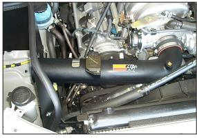
28. Install the K&N<sup>®</sup> intake tube onto the throttle body and align the tube with the saddle bracket.
