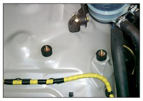
16. Install the two bumper studs into the original airbox mounting locations as shown.
