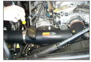
29. Secure the K&N<sup>®</sup> intake tube to the saddle bracket with the provided hose clamp. Also, tighten the hose clamp at the throttle body.
