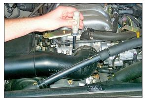
6. Loosen the hose clamp at the throttle body as shown.
