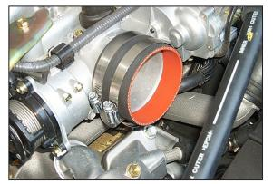
14. Apply the trim seal to the heat shield as shown above. Trim excess if needed.
