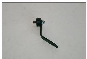
13. Assemble the angle bracket and the bumper stud with the provided hardware as shown above. Do not tighten completely.
