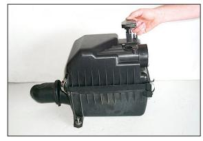
10. Remove the two screws that secure the mass air sensor then remove the mass air sensor as shown.
