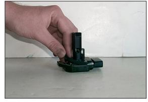
22. Apply the gasket to the mass air sensor, sticky side down as shown above.
