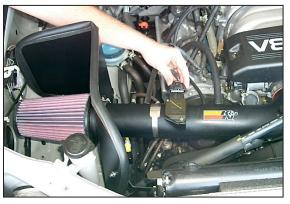
35. Re-connect the mass air sensor electrical connection.
