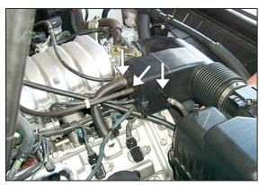
4. Remove the vent lines from the air intake resonator as shown.
