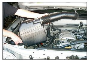
2. Loosen the two nuts that secure the throttle body cover then remove the throttle body cover
