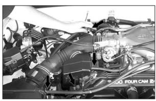
3. Disconnect the four vent hoses as shown above.
