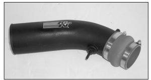
13. Install the 1/4" npt fitting onto the K&N $^{\! \rm B}$  intake tube as shown.
