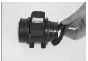
7. Remove the factory lip seal from the mass air sensor as shown.
