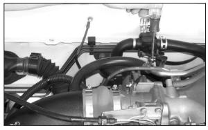
21. Remove the stock crankcase vent hose and replace it with the provided silicone hose and hose clamp. Secure it to the vent on the K&N® intake tube.
