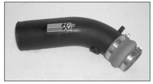
12. Install the silicone hump hose and hose clamps onto the  $K\&N^{\otimes}$  intake tube as shown.
