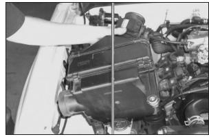
5. Loosen the three bolts that secure the air cleaner assembly then remove the air cleaner assembly as shown.
