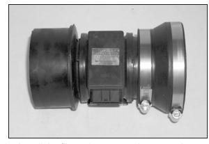
15. Install the filter adapter onto the mass air sensor as shown
