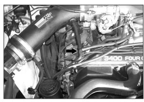
20. Install the rubber hose and vacuum "T" as shown.
