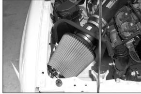
23. Install the K&N $^{\!0}$  air filter onto the filter adapter and slide the vent hose through the hole in the heat shield.
