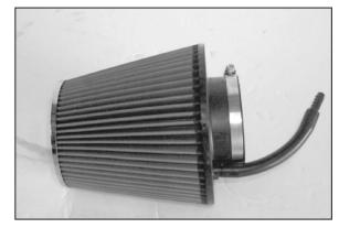
22. Install the vent hose with hose menders from step #19 into the K&N® air filter as shown.
