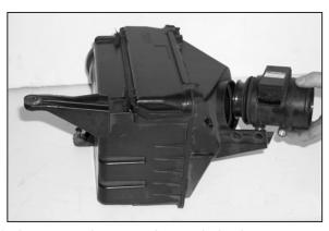
6. Loosen and remove the two bolts that secure the mass air sensor to the airbox, then remove the mass air sensor as shown.
