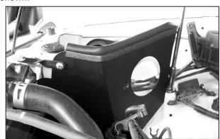
11. Using the provided hardware, secure the heat shield to the original air cleaner mounting holes
