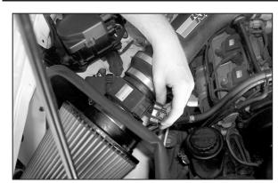
25. Reconnect the mass air sensor electrical connection as shown.
