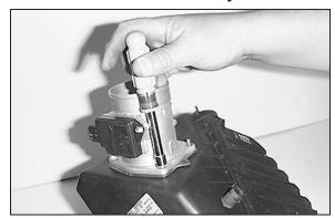
14. Loosen the 4 nuts and remove the mass air sensor from the airbox.
