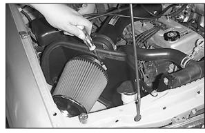
36. Install the air filter element and tighten the hose clamp.
