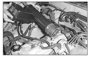
13. Loosen the hose clamp and remove the intake tube resonator assembly.
