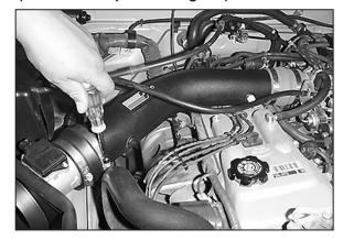
27. Install the intake tube and secure the hose clamp on the tube adapter.
