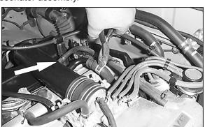
11. Disconnect the breather hose and A/C idle up magnetic valve vacuum line from the intake tube. Note: Not all vehicles are equipped with an A/C idle up magnet valve.
