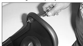
18. Attach the rubber mounted stud to the heat shield using the hardware provided.
