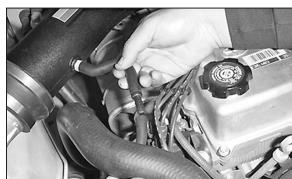
32. On models equipped with an evaporative canister vent line, connect the vent hose disconnected in step 5 to the 3/8"id vent hose using 3/8" hose mender provided. (Items U and Z in exploded diagram)
