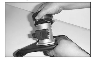
20. Install the tube adapter onto the flange of the mass air sensor and tighten hose clamp provided.
