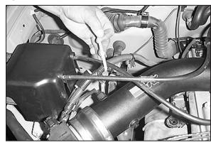
37. Secure the wiring harness to the throttle cable using the cable tie provided.
