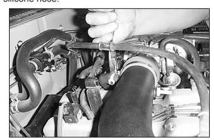
29. Attach the breather hose onto the vent on the intake tube.
