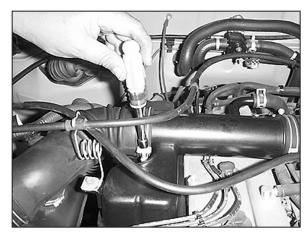
7. Loosen the hose clamp on the intake hose at the intake tube.
