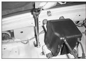
17. Attach the "L" bracket to the rear airbox mounting point using the hardware provided.
