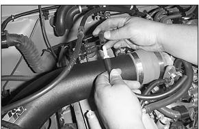
30. On models equipped with an A/C idle up magnetic valve vacuum line, connect the vacuum hose disconnected in step 11 to the 1/4"id vent hose using the 1/4" hose mender provided. (Items T and Y in exploded diagram).
