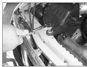
4. Loosen and remove the 3 bolts that retain the airbox.
