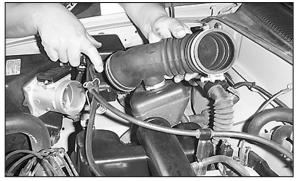
8. Detach the wiring harness and remove the intake hose.
