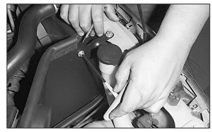
21. Install the heat shield assembly and secure to the brackets using the hardware provided.
