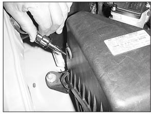
2. Remove the air temperature sensor from the airbox.
