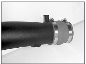
24. Install the silicone hose onto the  $K\&N^{\scriptsize @}$  intake tube.
