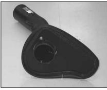
18. Secure the heat shield assembly to the K&N® intake tube with the provided hardware.
