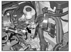
11a. On 2007 and later model vehicles, secure the tube mounting bracket assembly (070090).
