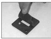
13. Install the provided gasket onto the K&N<sup>®</sup> mass air sensor adapter.
