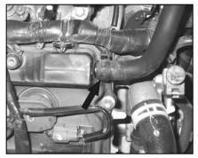
3. Release the spring clamp and disconnect the crank case vent hose.
