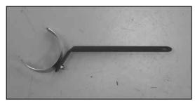
10. On 2004-2006 model vehicles, secure the saddle clamp to the tube mounting bracket (06489) with the provided hardware as shown.
