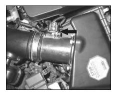
4. Disconnect the mass air sensor electrical connection.
