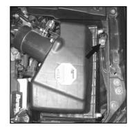
7. Remove the bolt that secures the air box to the inner fender.
