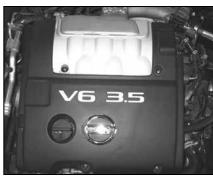
21. Re-install the engine cover and secure with the stock bolts.
