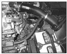
20. Install the provided crank case vent hose onto the vent port on the valve cover. Connect the open end to the  $\frac{1}{4}$ " NPT fitting installed into the K&N<sup>®</sup> intake tube.
