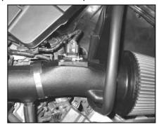
23. Re-connect the mass air sensor electrical connection.
