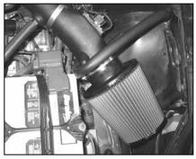
22. Install the K&N® air filter and secure with the
