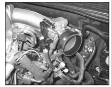
9. Install silicone hose (#08690) onto the throttle body and secure with the provided hose clamp.
