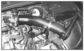
19. Install the K&N<sup>®</sup> intake tube assembly into the silicone hose at the throttle body and align with the saddle bracket installed in step #11. Secure the K&N<sup>®</sup> intake tube assembly with the provided hose clamps.
