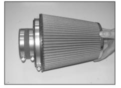
29. Install the filter adapter assembly into the  $K\&N^{\circledast}$  air filter.
