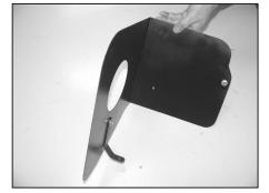
11. Install "L" bracket (07190) onto the heat shield as shown.
