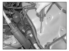
13. Using a screw driver, push the center of the plastic inner fender retaining clip through, then remove the clip from the inner fender.
