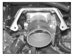
18. Install the provided silicone hose (08690) onto the throttle body with the provided hose clamps as shown.
