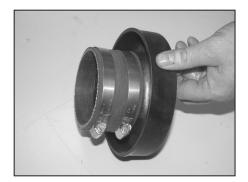
28. Install the provided silicone hose (#08630) onto the filter adapter as shown.
